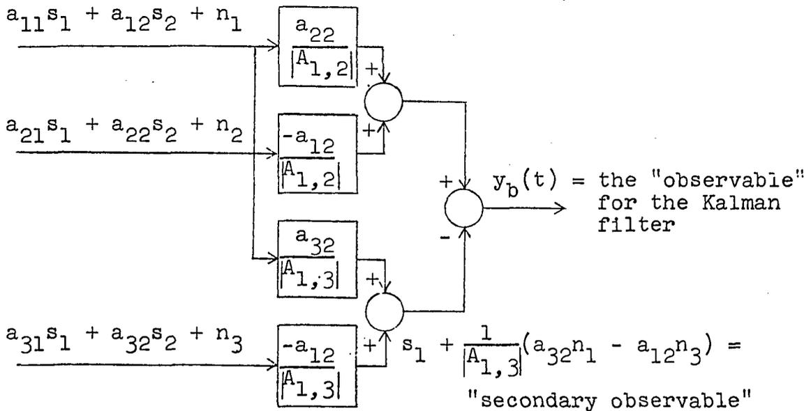
Figure 14. Linear, algebraic operator for "System b"
