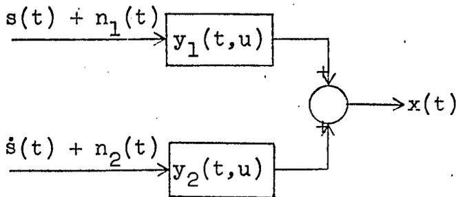
(b) The "optimum" distortionless filter
