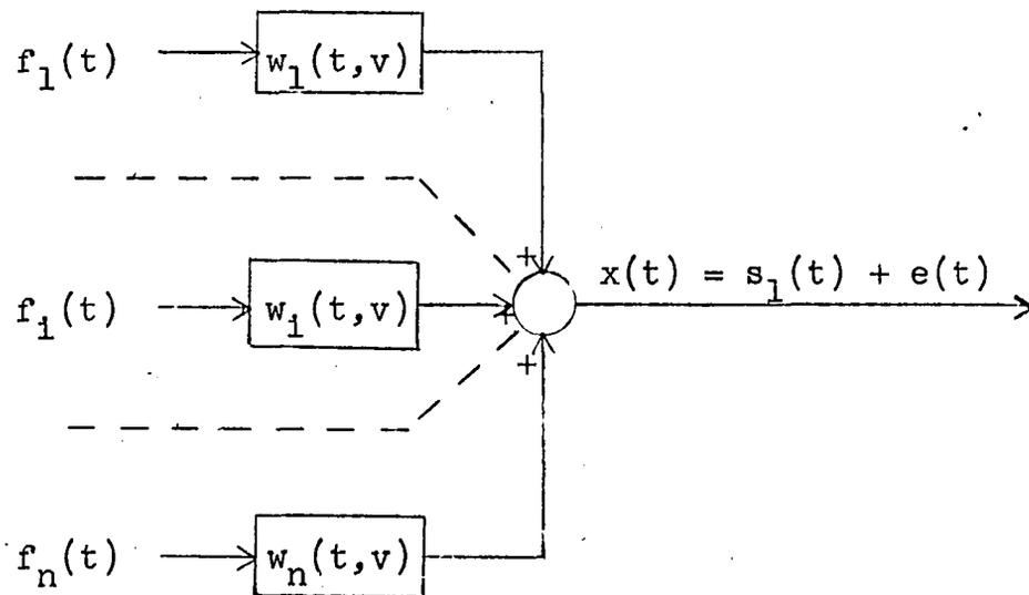
Figure 7. The general n-input, single output linear filter
