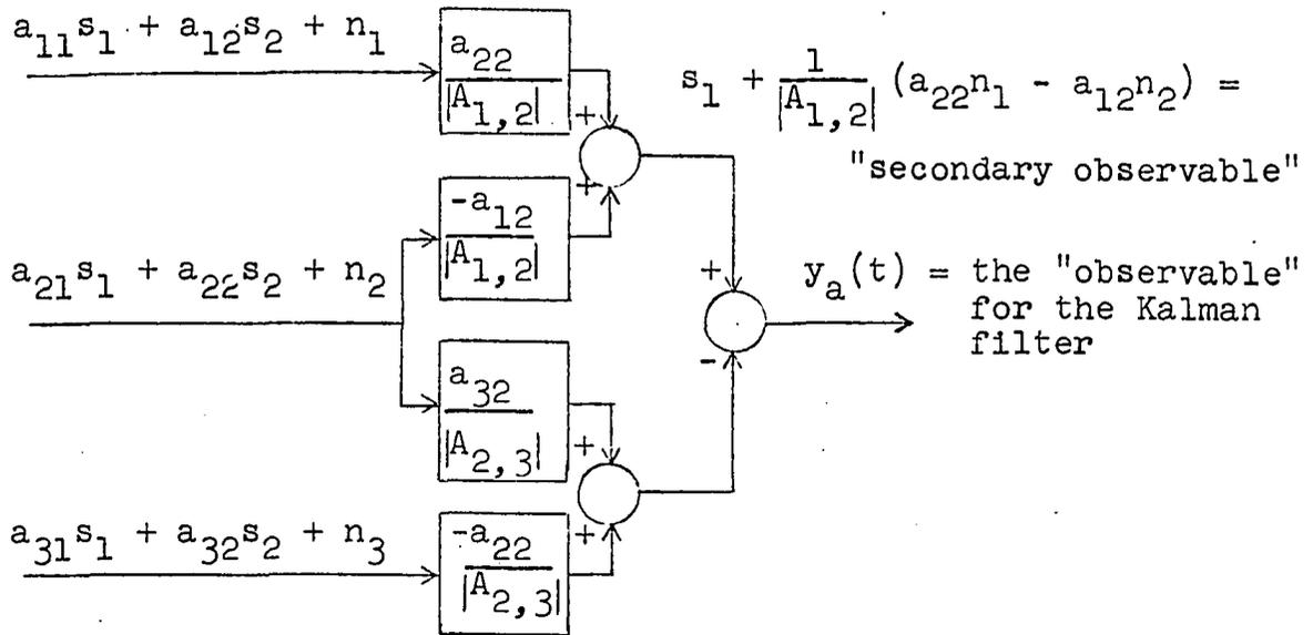
Figure 13. Linear, algebraic operator for "System a"
