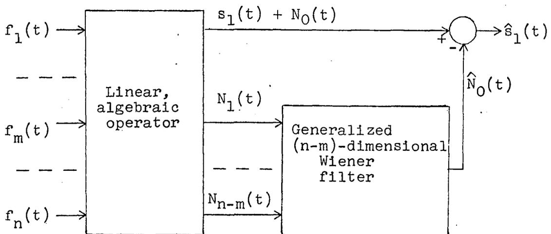
Figure 5. Block diagram of the "intuitive" system
