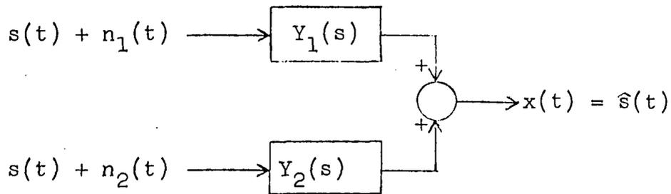
Figure 1. Linear system used to estimate  $s(t)$
